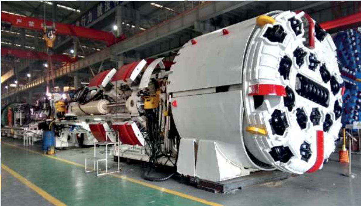
Tunnel boring machine
